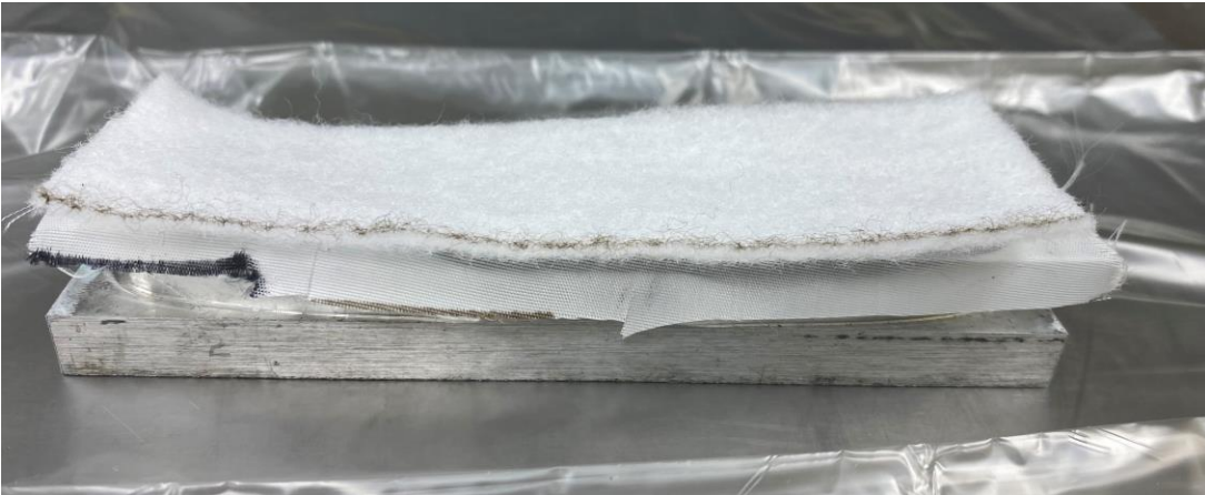
Composite layup on mold with breather layer
